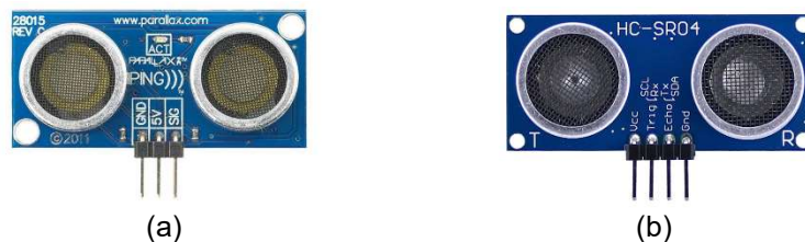
Figure 7.1: Types of pins on ultrasonic sensors from different manufacturers (a) 3-pin (b) 4-pin
