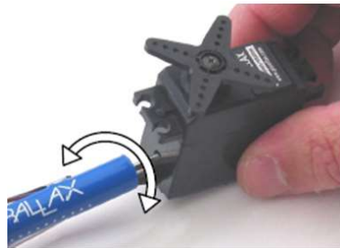
Figure 4.4: Adjusting the screw for servo motor centering (Source: parallax.com)
