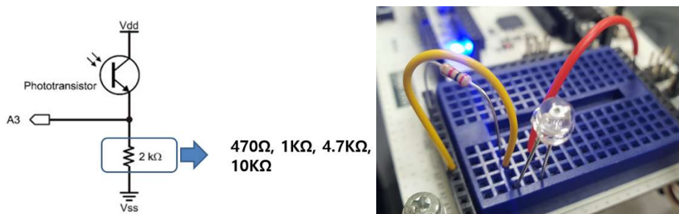
Figure 5.3: Analog Signal Processing Circuit for Phototransistor Light Sensor
