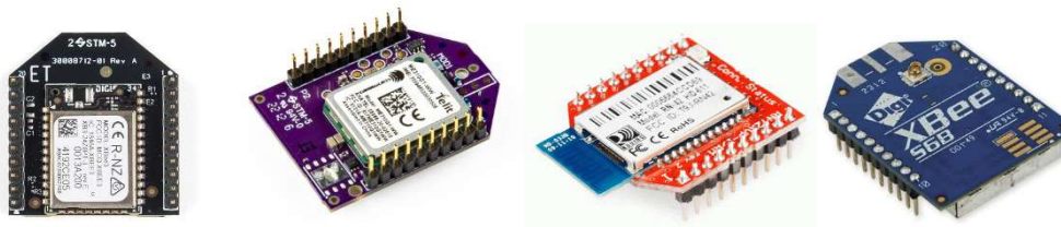
Figure 9.1: Types of XBee pin antennas to attach to the Arduino robot (abot)
